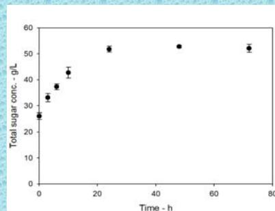
Figure 4. Time course of sugars release in bubble column after optimization of both laccases pretreatment (30 U/gbiomass, 15%w/v biomass loading, 60 nL/h, 24 h) and Cellic CTec2® hydrolysis (60 nL/h; 20 FPU/g cellulose).
