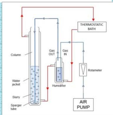
Figure 1. Schematic of the bioreactor set-up.
