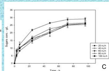
Figure 3. Hydrolysis profiles of apple pomace pretreated with laccase at different BL (A), LL (B) and AFR (C).
