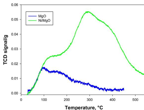
Fig. 9. Comparison of CO<sub>2</sub> TPD profiles of calcined MgO and Ni/MgO.
