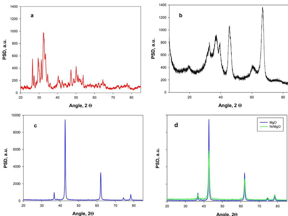
**Fig. 2.** XRD patterns of a) calcined HAP (red), b)  $\gamma$ - $\text{Al}_2\text{O}_3$  (black) and c) MgO (blue). D) Comparison between MgO and Ni/MgO (green). (For interpretation of the references to colour in this figure legend, the reader is referred to the web version of this article.)
