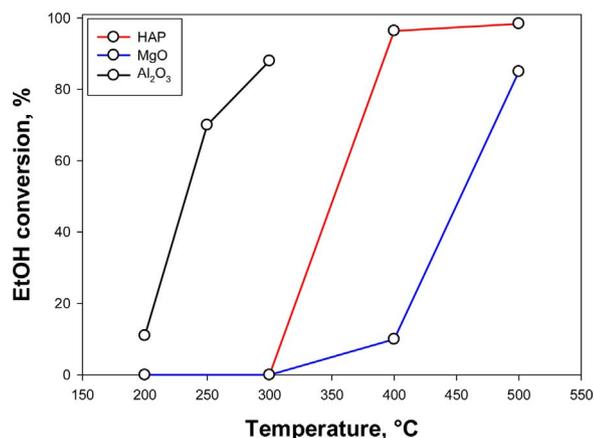
Fig. 5. Ethanol conversion as a function of temperature for HAP, Al<sub>2</sub>O<sub>3</sub> and MgO.
