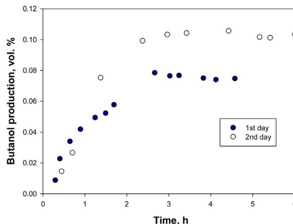
Fig. 10. Butanol production at 400 °C over Ru/MgO with time on stream. Comparison between results of the 1st day and those of the 2nd day under the same operation condition.
