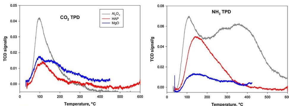
Fig. 3. CO<sub>2</sub> and NH<sub>3</sub> TPD profiles of calcined HAP,  $\gamma$ -Al<sub>2</sub>O<sub>3</sub> and MgO.
