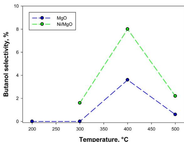
Fig. 7. Butanol selectivity as a function of reaction temperature for MgO and Ni/MgO.
