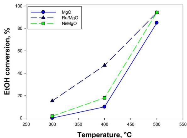
Fig. 6. Ethanol conversion as a function of temperature for MgO, 0.16% Ru/MgO and 0.47% Ni/MgO.
